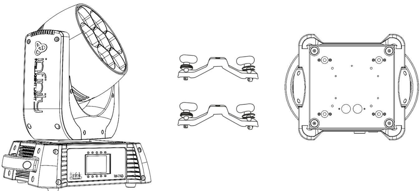
The Infinity can be placed on a flat stage floor or mounted to any kind of truss with a clamp.
