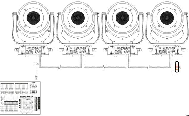
Note: Link all cables before connecting electric power
