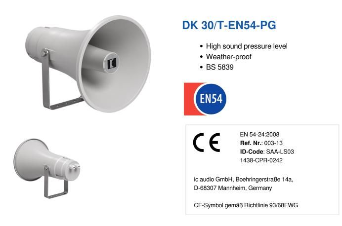
The 30W powered speaker is equipped with a 100V line transformer with 4 power adjustments, also lowimpedance operation (20 ohm) is possible. The impact-resistant ABS housing UL94V0 in RAL 7035 guarantees long-term stability. For additional reliability, a ceramic block and a thermal fuse is provided.
